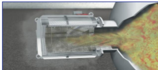
The flame gases, which can reach temperatures of up to 1,500°C, are cooled down in a special stainless steel mesh filter cage. This reduces the volume of gas that escapes, and thus extinguishes the flame. (Fig. C)
