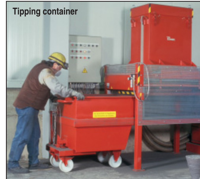
Trolley with tipping mechanism
